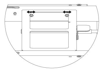
Push the tray to the left or the right, align the outside of the legs with the head of the tabletop.
