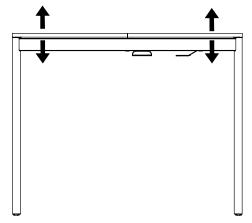
With the leveler you can adjust the outside of the extension leaf to the correct height.
