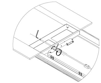
Loosen the 3 bolts so you can move the axle.
