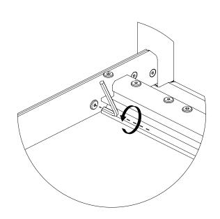
Loosen the 2 bolts to push out the legs. Tighten the 2 bolts to push the legs inwards. Align the legs with the edge of the tabletop.
