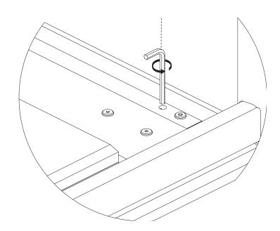
Loosen the bolt under the profile to push the tabletop up.
