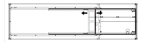
When the substructure is in the right shape, fix the bolts while pushing the tray in the correct position.
