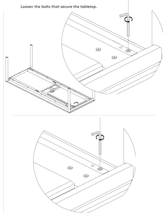
When the correct height is reached, secure the tabletop with the other bolt.
