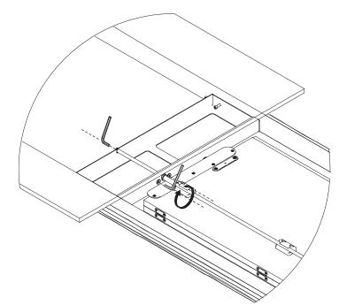
Tighten the 3 bolts while holding the axle in place.
